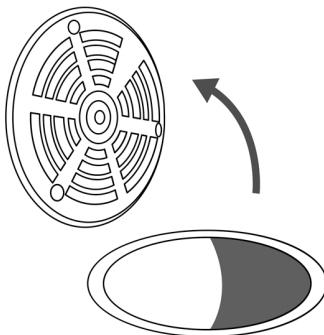
2. Press the Green Drain trap into the drain pipe so that it is in the same level with the top edge of the pipe.
